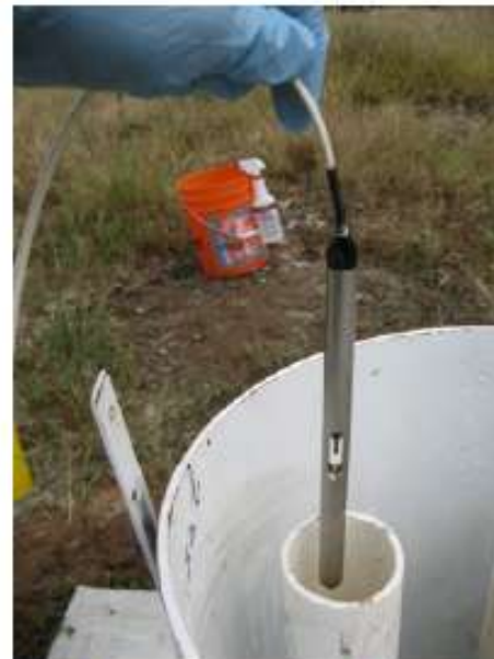
Electric water-level sander used to measure the depth-to-static-groundwater in a monitoring well
