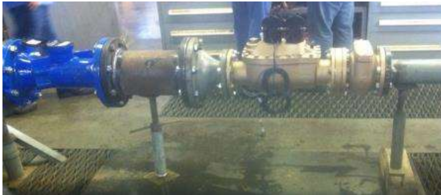
Ultrasonic meter installed on WV test bench
